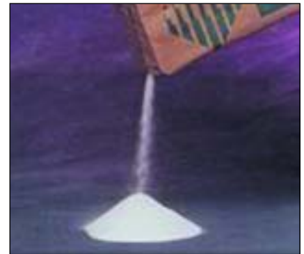
Sodium bicarbonate, also known as baking soda, is a water-soluble abrasive. Photos above courtesy of Armex®
