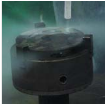
Dry ice sublimates during blasting, going from a solid directly to a gas.
