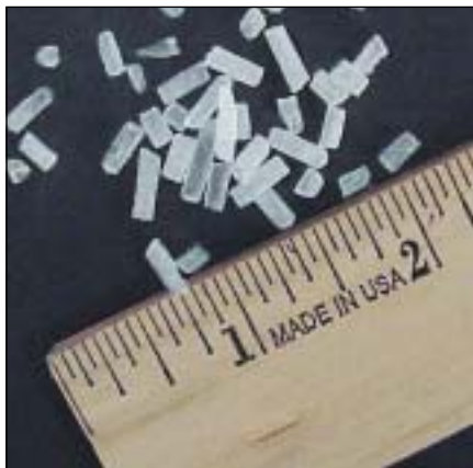
Dry ice particles vary to about \frac{1}{8} in. (3 mm) Photos above courtesy of Cold Jet, Inc.
